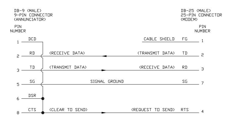
PINS NOT LISTED ARE NOT USED FOR THIS APPLICATION AND ARE LEFT OPEN.
