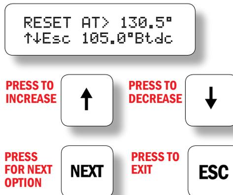
**NOTE:** Adjustment of this parameter should be done while individual cylinder offsets are all at zero.
