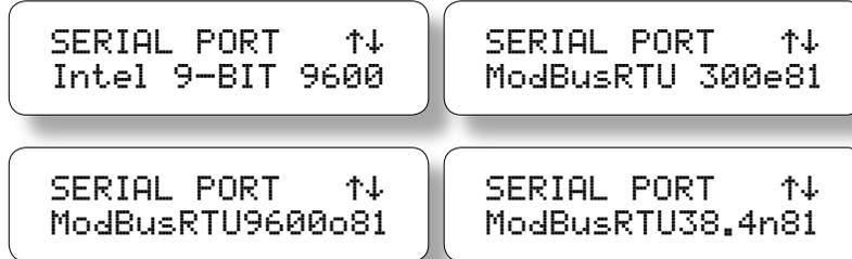
**9.8** From the next setup screen the communication ID-Code or Node-ID can be viewed or modified. Suitable ID-Codes for ModBus are (1 to 247), while suitable ID-Codes for the standard Intel 9-bit communication format are (1 to 254). Use the arrow keys to select the Node-ID.
