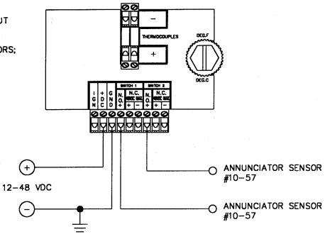
NORMALLY CLOSED OUTPUT SWITCH WITH ALTRONIC ANNUNCIATOR USING NORMALLY CLOSED SENSORS; DC-POWERED.
