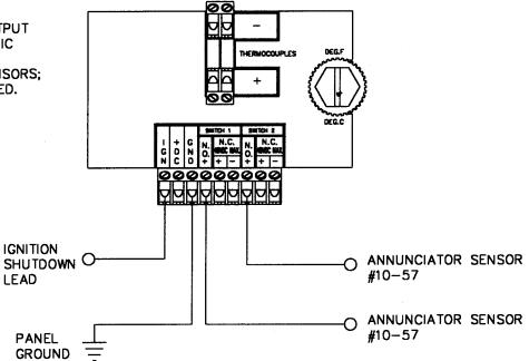
NORMALLY CLOSED OUTPUT SWITCH WITH ALTRONIC ANNUNCIATOR USING NORMALLY CLOSED SENSORS; C.D. IGNITION POWERED.
