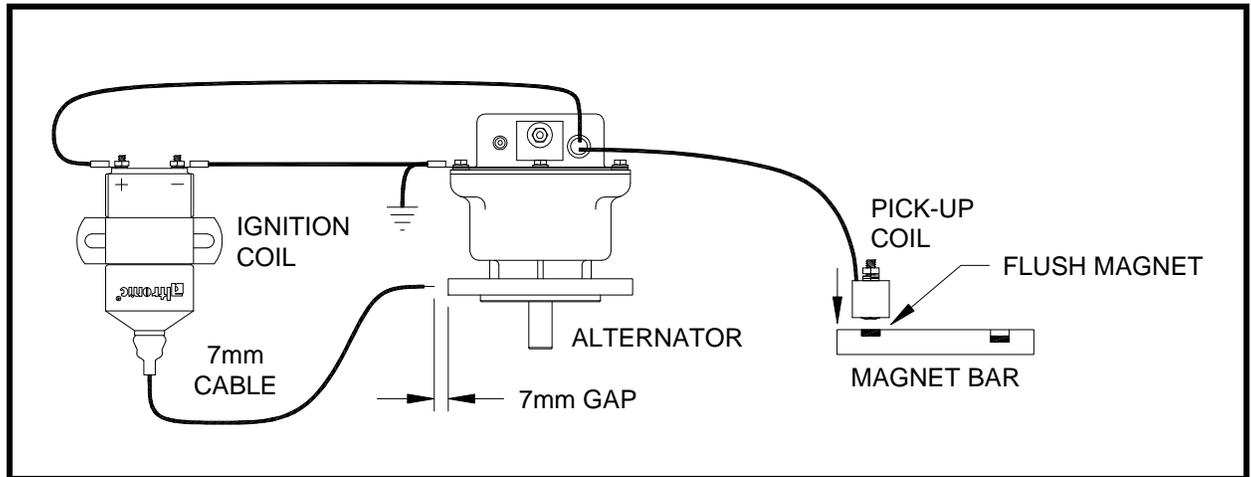
B. Connect the voltmeter to the electronic box as indicated below; turn the alternator shaft one or more revolutions by hand:
