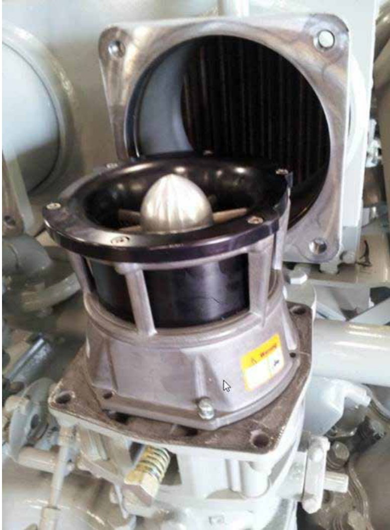
Figure 8: Properly seated venturi assembly.
