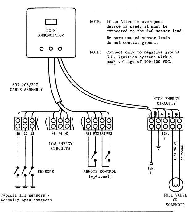
WARNING: Sensor leads from the annunciator MUST NOT CONTACT any external voltage source. Damage to the system will result from connection between the sensor leads and the ignition system or any AC or DC power source.
