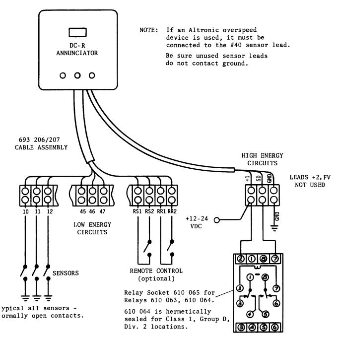
Relay contacts shown in the normal run (energized) state. Contact state is the opposite on a fault signal or loss of 12-24 VDC power.
