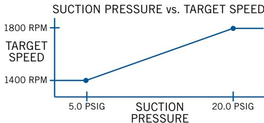
The permissive channel can be any channel from 20 to 27, and is not limited to suction pressure.
