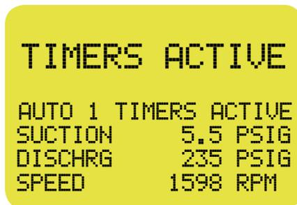
MANUAL MODE with the engine running and timers expired.
