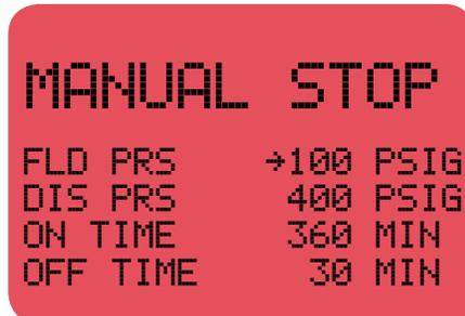
The user presses the ENTER key to move the cursor adjacent to the value to be changed, and then uses the UP and DOWN arrow keys to adjust the values. AUTO 4 combines the AUTOSTART features of AUTO 1, AUTO 2 and AUTO 3.
