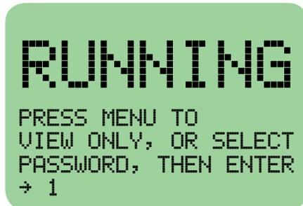
Press the MENU key again to view menu parameters and not modify them. Press the UP, UP/TENS, DOWN, DOWN/TENS keys to modify the value to the correct password value. If the password is not correct, the display shows the first MENU screen but does not allow for values to be modified. If the password is correct, the following MENU will appear:
