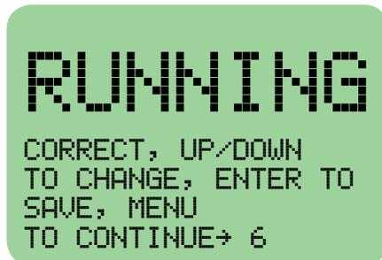
The password may be changed at this point, or the user can continue to the MENU to view and modify menu parameters. Use the UP, UP/TENS, DOWN, DOWN/TENS key to modify the new password value and press ENTER to save the new password.
