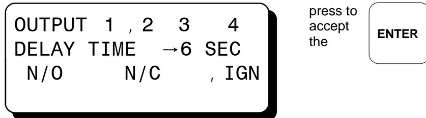
The selection arrow replaces the diamond indicating a change can be made. The selected output switch can be configured for N/O (normally open), N/C (normally closed), or IGN (ignition module 691124).
