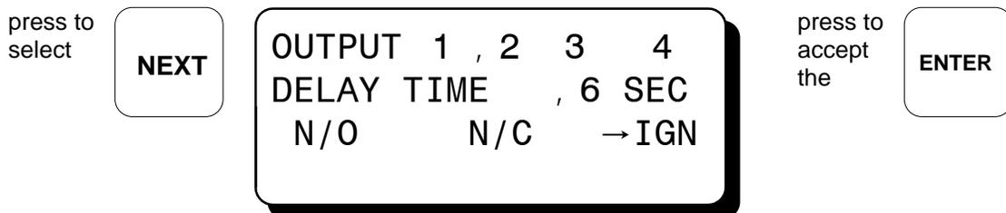
Upon pressing the ENTER key, a diamond will replace the selection arrow. To view or edit the next output number, press the NEXT or →TENS or ←TENS keys until the arrow points to the desired output number and repeat the process.
