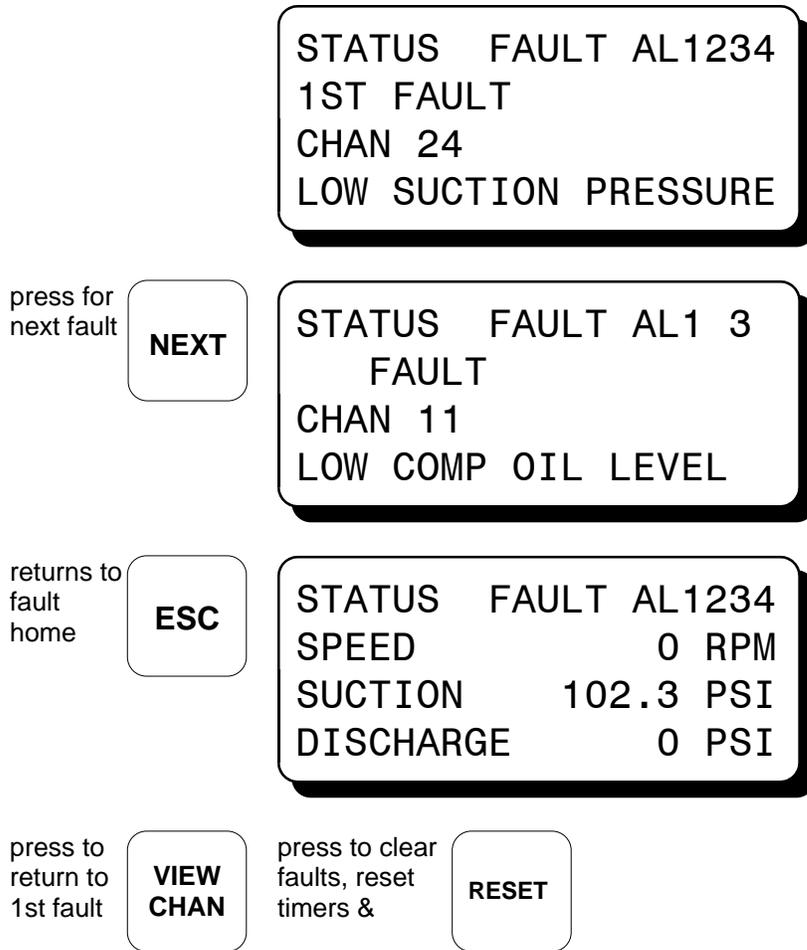
NOTE: The reset function can also be implemented by using the external RESET input available on the Terminal Module. The behavior of the Annunciator and display will be identical to that obtained by pressing the local RESET key on the Display Module.
