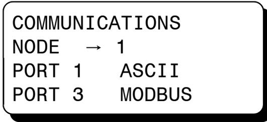
Use the NEXT key to select node, port1 or port 3; then use the UP or DOWN arrow keys to change the node number from 1 to 99 and port 1 and port 3 from ASCII to MODBUS. Press ENTER to save selection.
