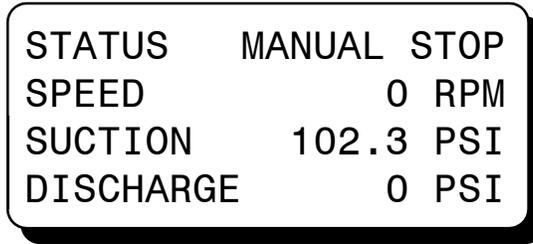
NOTE: The stop function can also be implemented remotely by using the external STOP input available on the Terminal Module. The behavior of the Annunciator and display will be identical to that obtained by pressing the local STOP key on the Display Module.
