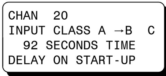
The selection arrow will point to the current class B time. To adjust it, use the ↑UNITS or ↓UNITS keys to increase or decrease the value by one or use the →TENS or ←TENS keys to increase or decrease the value by ten. Once the desired time is displayed, press the ENTER key to save the new value.
