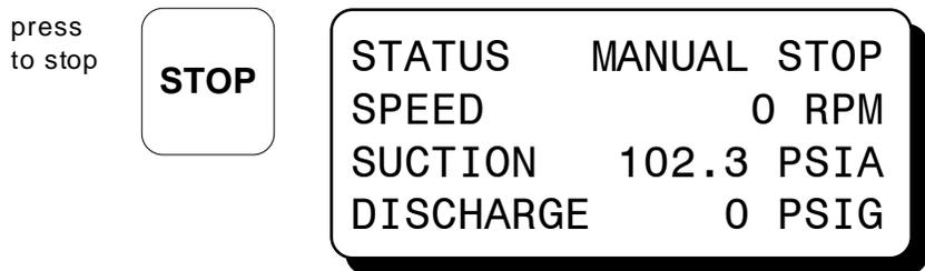
NOTE: The stop function can also be implemented remotely by using the external STOP input available on the Terminal Module. The behavior of the Controller and display will be identical to that obtained by pressing the local STOP key on the Display Module.
