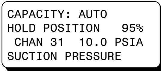
Indicates that the current value of channel 31 which is the Primary control setpoint is within the allowable deadband of the controller and no controller output change is being made at this time.
