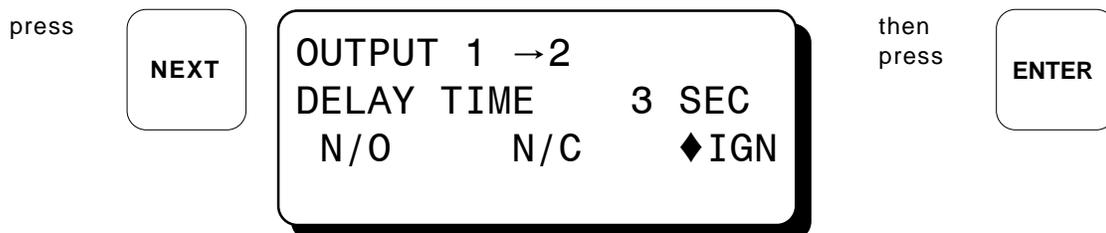
A diamond will replace the arrow in front of the selected output switch. An arrow will proceed the delay time indicating a change can be made to the selected output's delay time. Use the ↑UNITS or ↓UNITS keys to increase or decrease the value by one or use the →TENS or ←TENS key to increase or decrease the value by ten. The ENTER key accepts the change and advances the pointer to select either N/O, N/C or IGN.
