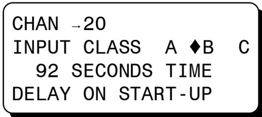
To view the next channel number, press the NEXT key until the arrow points to the channel number. Select another channel number by using the ↑UNITS or ↓UNITS keys to increase or decrease the channel by one or use the →TENS or ←TENS key to increase or decrease the channel by ten and press ENTER.
