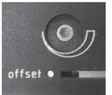
With this view, **turn counter-clockwise (increasing thickness) to increase outlet pressure.**
