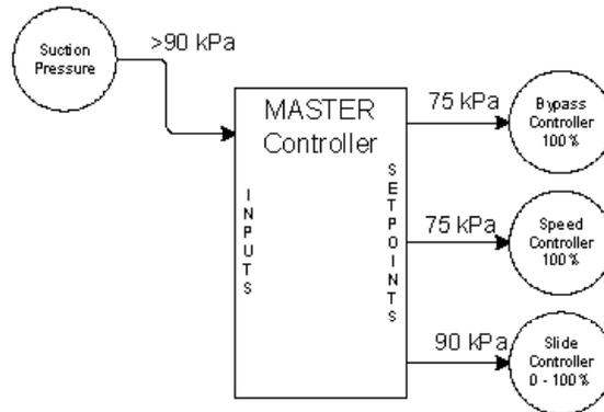
Using the same initial conditions—slide 100%, speed 100% and bypass 100% closed. If the Manifold pressure increases above setpoint the MC would insert the setpoint for the manifold pressure into the slide controller. The speed and bypass valve controllers would receive the manifold pressure setpoint plus the offset for the manifold pressure. The same sequencing will occur to attempt to control the manifold pressure at setpoint.
