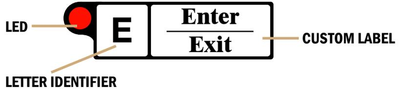
While the key is pressed, the **LED** will illuminate. It will normally go out as soon as the key is released. If it doesn't go out the computer is performing some function, an error has occurred, or in some cases it may be programmed to stay on or flash. For example, **LED** for key **1/Reset**, will normally be programmed to flash whenever a shut-down occurs and it will continue to flash until the problem has been cleared and the key is pushed.
