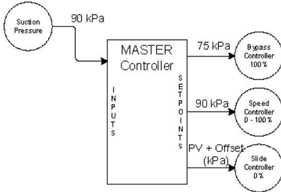
The speed will be manipulated to attempt to maintain suction pressure at the setpoint of 90kPa. With the offsets applied to the controllers as shown above it is clear how the MC sequences the controllers. The only time more than one controller will be changing its controlled variable will be if the suction pressure was to decrease rapidly below the actual setpoint minus the offset, for our example 75kPa. At this point, both speed and bypass valve would be reacting to changes in suction pressure:
