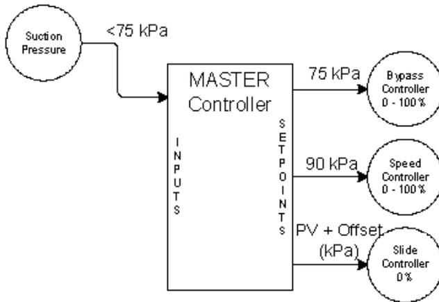
If the suction pressure began to increase, the unit would begin loading. Starting with the controller currently being controlled and sequencing through the controllers. For example, if the speed is being manipulated to maintain suction at 90kPa the setpoints in the three controllers would be as follows:
