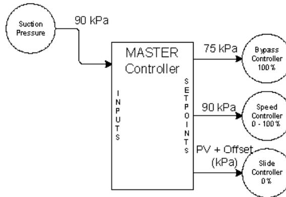
The speed would continue to increase to attempt to maintain suction pressure at 90kPa. Once the speed controller output increased to 100%, the next controller, in this case the slide valve controller, would get the actual setpoint and the speed controller would get a setpoint equal to the actual minus the offset value:
