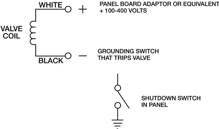
**DC Powered (Failsafe) Model 690045-1:**
