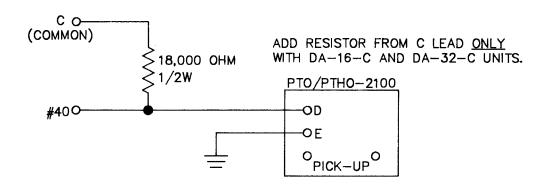
NOTE: #40 SENSOR OF THE DA/DC ANNUNCIATOR MUST BE USED FOR OVERSPEED WITH AN ALTRONIC PTO/PTHO DEVICE.
