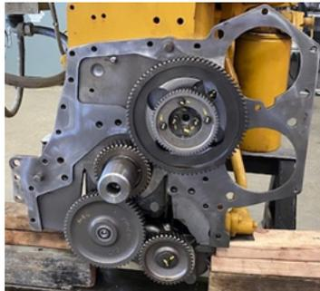
Cover removed showing original cam trigger gear
