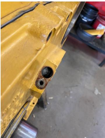
Cam Pickup Mounting Hole
