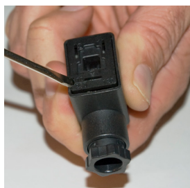
FIGURE VIII Removal of Connector Back Shell
