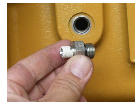
FIGURE V Manifold Adapter Installation
