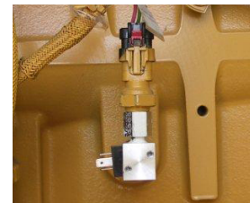
FIGURE VII Manifold Sensor and Harness installed on Sensor By-Pass Kit Assembly
